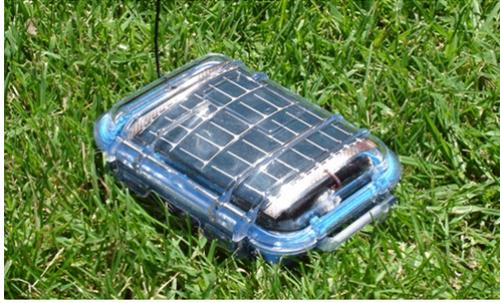
Figure 2.1: The heliomote prototype node [5].
