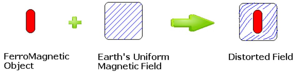
Figure 3.1 Earth's magnetic field and effect of Ferrous object on it
