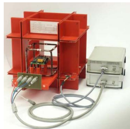
Figure 2.12 Sensor sensitivity estimating by Helmholtz coil [24]
